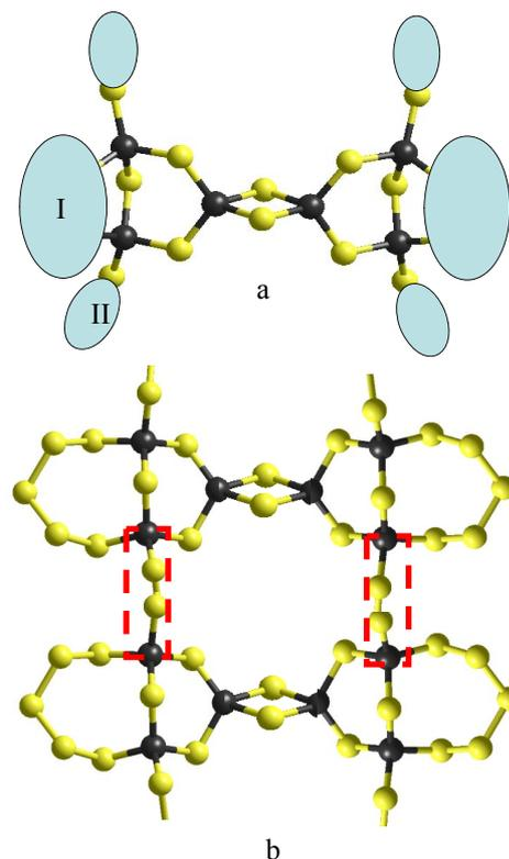
**Figure 2** Outtrigger raft structural motive in  $Ge_xSe_{100-x}$  glasses within  $20 < x < 28$  compositional range (a) and most energetically favourable connection for optimally-constrained  $Ge_{21.5}Se_{78.5}$  composition (b). Area I denotes the place of initial Se-Se dimers, area II shows a place of inter-cluster bridges (denoted also by red dashed rectangle). Black four-fold coordinated spheres denote Ge atoms, two-fold coordinated yellow – Se atoms.
