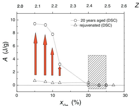
**Figure 4** Areas  $A$  under the endothermic peaks of DSC curves recorded with 5 K/min heating rate for aged and rejuvenated  $\text{Ge}_x\text{Se}_{100-x}$  glasses. Cross-hatched area shows the reversibility window determined in [14].
