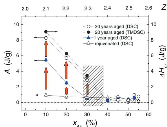
**Figure 3** Areas  $A$  under the endothermic peaks of DSC curves recorded with 5 K/min heating rate for aged and rejuvenated  $\text{As}_x\text{Se}_{100-x}$  glasses. TMDSC  $\Delta H_{nr}$  values are taken from [15] for comparison. Cross-hatched area shows the reversibility window determined in [13].
