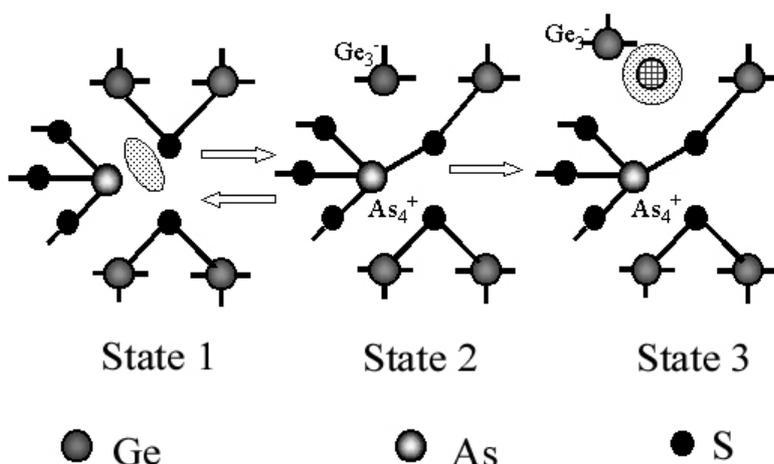
**Fig. 1** Topological scheme of the main bond-switching reaction in  $v$ - $\text{As}_2\text{S}_3$ - $\text{GeS}_2$ , accompanied by the separation of CTDs with an additional open-volume microvoid.
