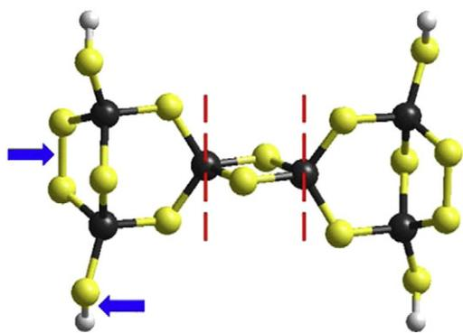
**Fig. 1.** Fragment of  $\text{Ge}_{30}\text{Se}_{70}$  glass structure (black – four-fold coordinated Ge atoms; yellow – two-fold coordinated Se atoms) forming ORR structural motive of two ES– $\text{GeSe}_{4/2}$  and four CS– $\text{GeSe}_{4/2}$  tetrahedra terminated by Se–Se dimers. The places, where the extra Se atoms can be incorporated, are shown by arrows; two side-ORR and one central-ORR parts are distinguished by dashed lines.
