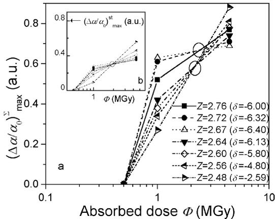
Fig. 3. Dose dependences of radiation-stimulated maximal relative changes of absorption  $(\Delta\alpha/\alpha_0)_{\max}$  for  $\text{As}_2\text{S}_3\text{-Ge}_2\text{S}_3$  glasses: a – the total effect, b – the static effect ( $\delta$  – atomic compactness [4]).
