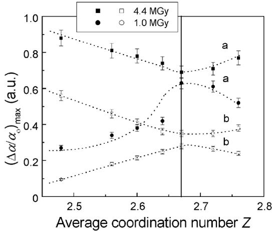
Fig. 1. Compositional dependence of total (curves a) and static (curves b) radiation-induced changes for  $\text{As}_2\text{S}_3$ - $\text{Ge}_2\text{S}_3$  glasses  $\gamma$ -irradiated with 1.0 and 4.4 MGy absorbed doses.
