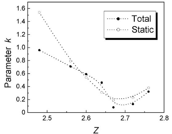
Fig. 4. Compositional dependences of parameter  $k$  from formula (3) in the investigated  $\text{As}_2\text{S}_3\text{-Ge}_2\text{S}_3$  glasses.
