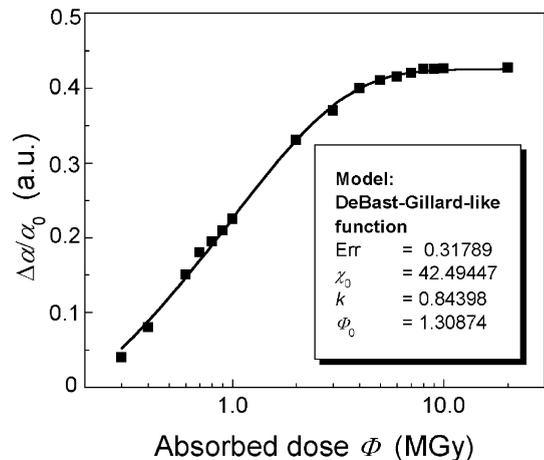
Fig. 2. Dose-dependence of  $\gamma$ -induced optical changes (registered at 600 nm wavelength) in vitreous  $\text{As}_2\text{S}_3$  irradiated with  $\sim 5$  Gy/s dose power and fitting parameters according with curve obtained from formula (3).
